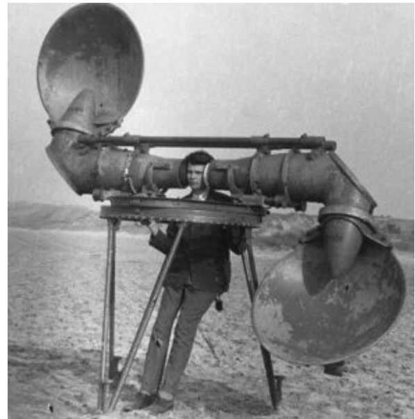
A 1920s aircraft detector
